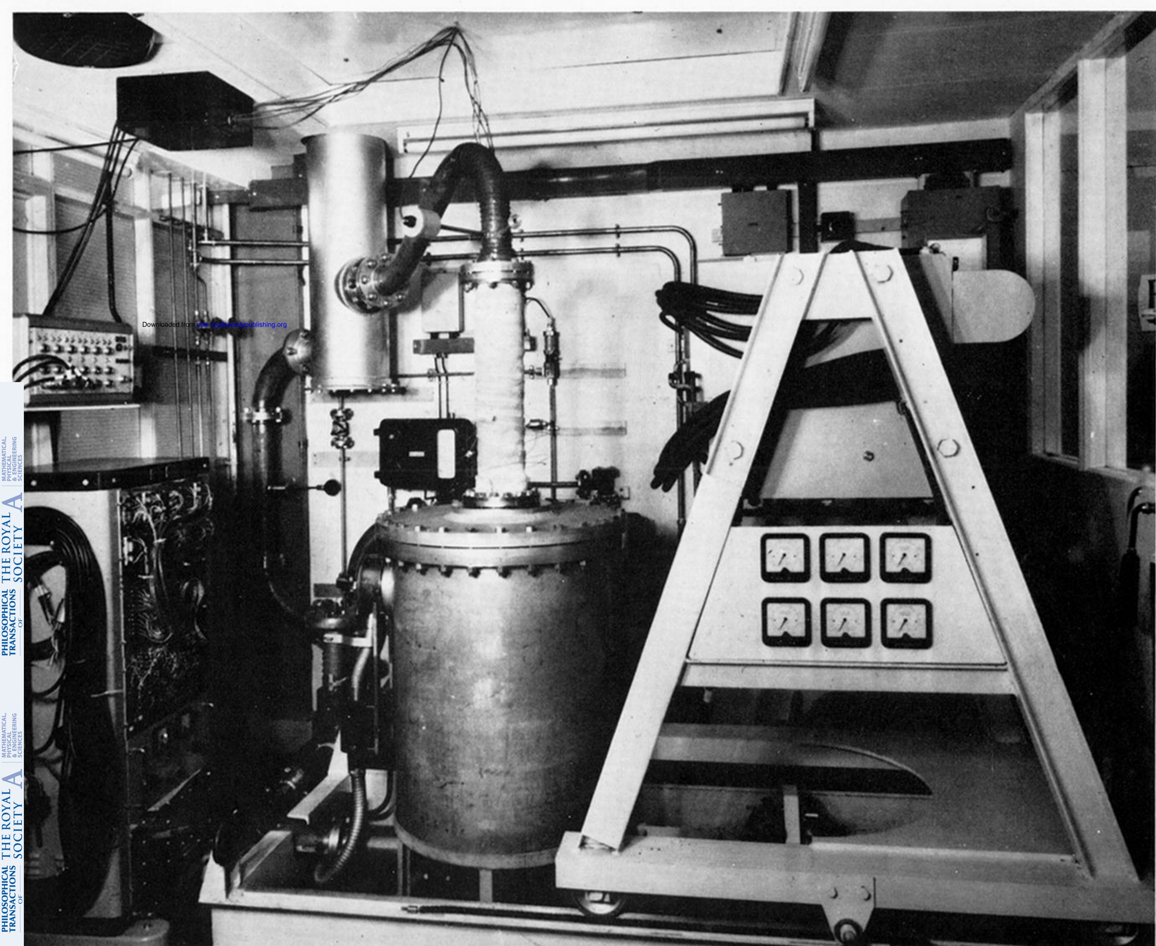
FIGURE 17. A.E.R.E. blow-down argon-potassium m.p.d. rig.
